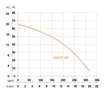
Shaft Speed: 3450 rpm Outlet: 80mm, 3in
